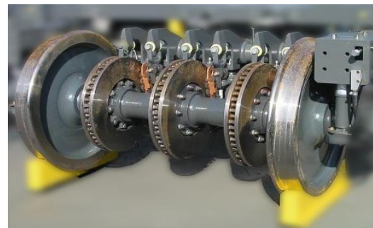
Fig. 1. Wheel-mounted ventilated brake discs used in high-speed train
